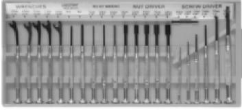
**POCKET JEWELLERS SCREWDRIVER SET** a 4 piece miniature screwdriver set that features a quality handle with swivel cap and 3 double ended drivers. The blade sizes included are flat 1.5, 2.0, 3.0 and 3.5mm, and No0 and No1 crosspoint. Supplied in a plastic storage case.
